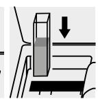
Place the cell into the cell compartment.
