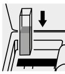
Place the cell into the cell compartment.
