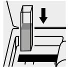
Place the cell into the cell compartment.
