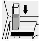
Place the cell into the cell compartment.
