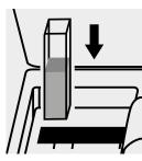
Place the cell into the cell compartment.
