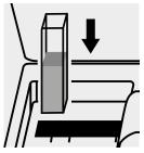
Place the cell into the cell compartment.
