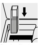
Place the cell into the cell compartment.
