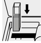
Place the cell into the cell compartment.
