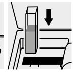
Place the cell into the cell compartment.
