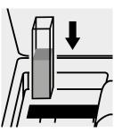
Place the cell into the cell compartment.
