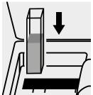
Place the cell into the cell compartment.
