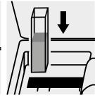
Place the cell into the cell compartment.
