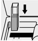
Place the cell into the cell compartment.
