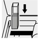
Place the cell into the cell compartment.
