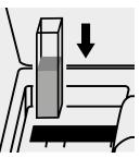
Place the cell into the cell compartment.
