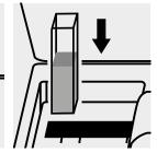
Place the cell into the cell compartment.
