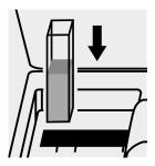
Place the cell into the cell compartment.
