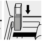
Place the cell into the cell compartment.
