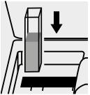
Place the cell into the cell compartment.
