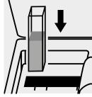
Place the cell into the cell compartment.
