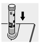
Place the cell into the cell compartment. Align the mark on the cell with that on the photometer.
