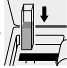
Place the cell into the cell compartment.
