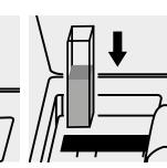
Place the cell into the cell compartment.
