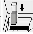
Place the cell into the cell compartment.
