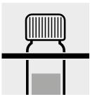
Remove the cell from the thermoreactor and place in a test-tube rack to cool.
