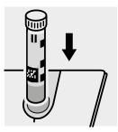
Place the blank cell into the cell compartment. Align the mark on the cell with that on the photometer.
