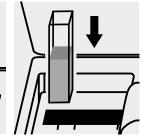
Place the cell into the cell compartment.
