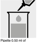
Pipette 0.50 ml of  $H_2O_2$ -1 into a test tube.
