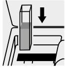
Place the cell into the cell compartment.
