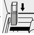
Place the cell into the cell compartment.
