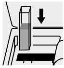
Place the cell into the cell compartment.
