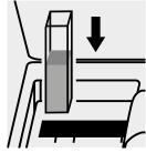
Place the cell into the cell compartment.
