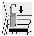
Place the cell into the cell compartment.
