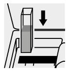
Place the cell into the cell compartment.
