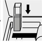
Place the cell into the cell compartment.
