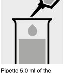
sample into a test tube.
