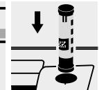
Select method with AutoSelector measuring range 5 - 150 mg/l NH<sub>4</sub>-N.
