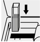
Place the cell into the cell compartment.
