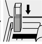
Place the cell into the cell compartment.
