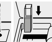
Place the cell into the cell compartment.
