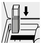
Place the cell into the cell compartment.
