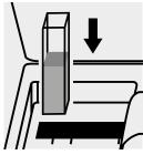
Place the cell into the cell compartment.
