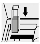
Place the cell into the cell compartment.
