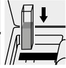
Place the cell into the cell compartment.
