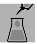
Acidify a portion of the extract with **hydrochloric** acid 2 mol/l Titripur<sup>®</sup> (Cat. No. 109063) (0.3 ml per 100 ml of extract).
