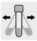
Shake the cell **vigorously for 5 seconds** to dissolve the solid substance.
