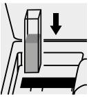
Place the cell into the cell compartment.
