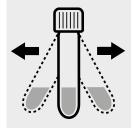
Shake the cell vigorously for 30 seconds. Leave to stand to allow phases to separate.
