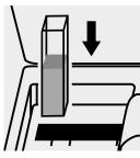
Place the cell into the cell compartment.
