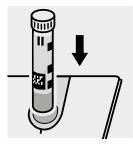
Place the cell containing the sample into the cell compartment. Align the mark on the cell with that on the photometer.
