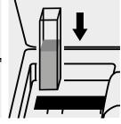
Place the cell into the cell compartment.
