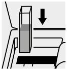
Place the cell into the cell compartment.
