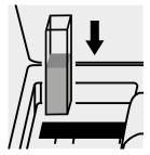
Place the cell into the cell compartment.
