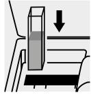
Place the cell into the cell compartment.
