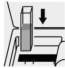
Place the cell into the cell compartment.
