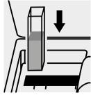
Place the cell into the cell compartment.
