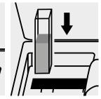
Place the cell into the cell compartment.
