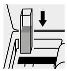
Place the cell into the cell compartment.
