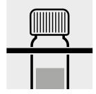
Remove the cell from the thermoreactor and place in a test-tube rack to cool to room temperature: pretreated sample.
