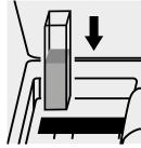
Place the cell into the cell compartment.
