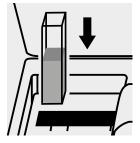
Place the cell into the cell compartment.
