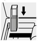
Place the cell into the cell compartment.
