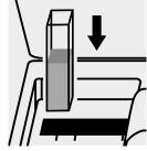
Place the cell into the cell compartment.
